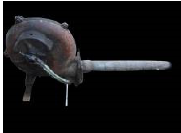
Fig. 9: Handle bellows use by the Gadulia Lohar, Hiranmagri road.
